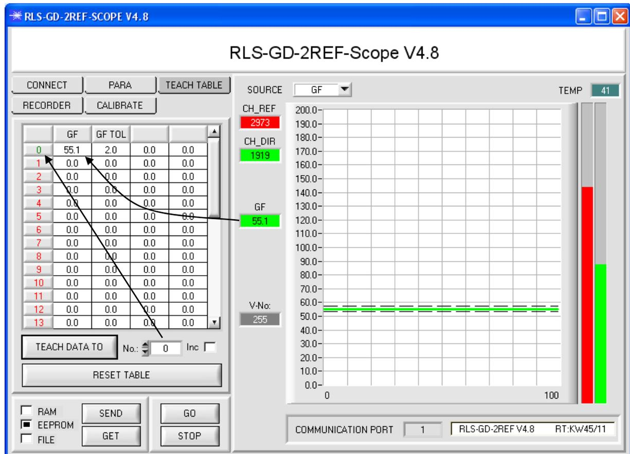
Now press the **SEND** button to inform the sensor about the taught vector. Then activate the **GO** mode again. When the sensor recognises a row vector, the corresponding row number is visualised under **V-No.:**. A value of 255 means that none of the taught vectors were recognised.
